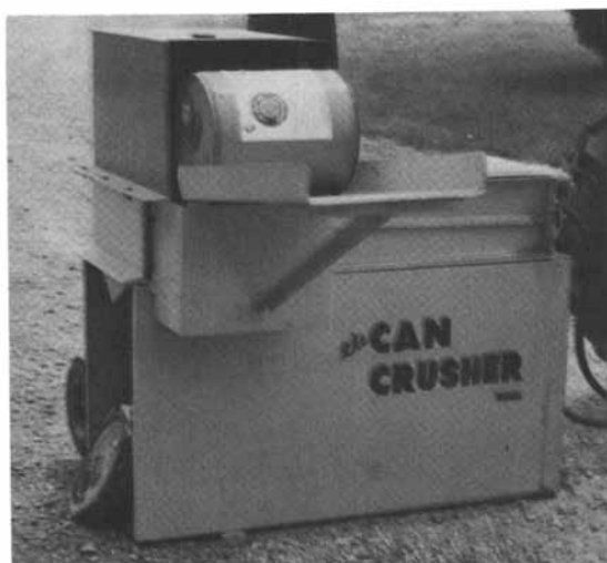
Figure 3. Hydraulically operated can crusher with five gallon cans before and after crushing.
